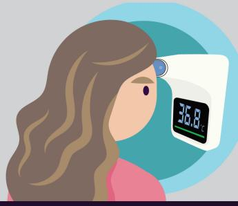
When you hear a long beep the measurement has finished. It will display a rotating bar, you will notice the device will count up to 5.
